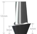
Use to fabricate cement-retained, single- or multiple-unit prostheses. Packaged with an abutment screw (130-300 or 140-300). Titanium Alloy. Final torque: 30Ncm.
